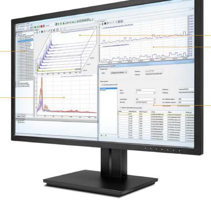
Real time visualization of the spectra as an individual spectrum, waterfall or contour view
