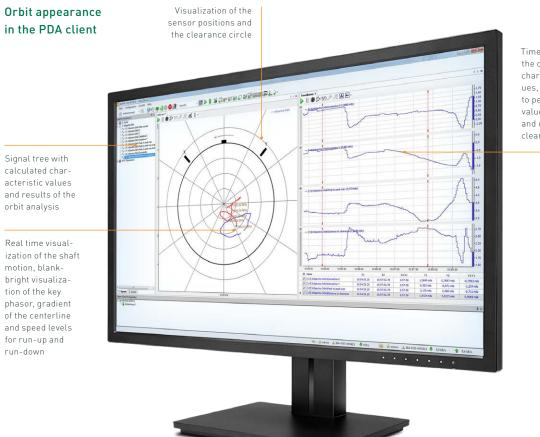
Time gradient of the calculated characteristic values, such as: peak to peak maximum value, eccentricity and distance to the clearance circle Success story
