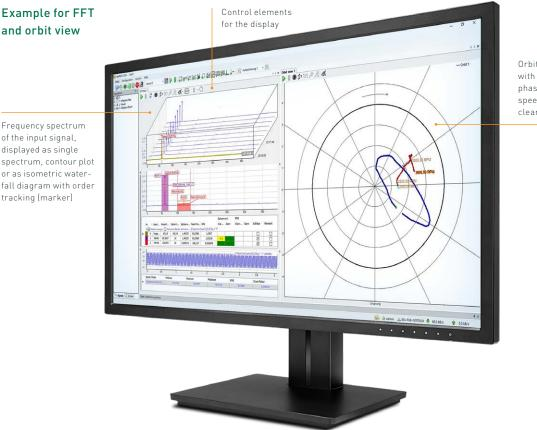
Orbit display with orbit, key phasor, centerline, speed stages and clearance circle.
