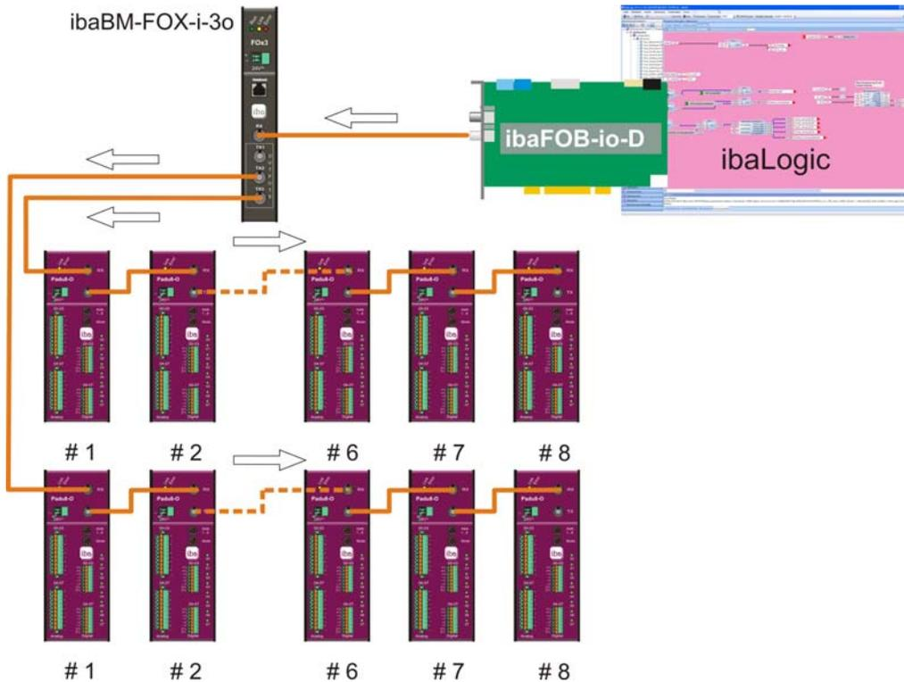
Figure 6: Process IO redundancy
